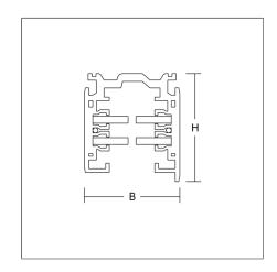
Aluminium extrusion profile painted, tracks can be cut to any required length, may be used within hand's reach, with integrated additional 2-pole DALI cable, supply cable 16A / 400V, control cable DALI 2x1A / 50V FELV AC.
