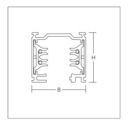
Aluminium extrusion profile painted, tracks can be cut to any required length, may be used within hand's reach, with three mounting holes at 100, 990, 1880mm.
