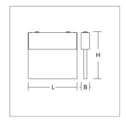
Luminaire for escape route identification. Housing: extruded aluminium profile, anodised or powder-coated. Display panel: highly transparent panel, plastic, with legend on one side/both sides. Electronic ballast included. Self-contained system with automatic self-test. Please indicate legend number when placing your order!
