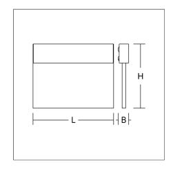
Luminaire for escape route identification. Housing: extruded aluminium profile, anodised or powder-coated. Display panel: highly transparent plastic, with motifs on one side. Electronic ballast included. Self-contained system with automatic self-test. Please indicate legend number when placing your order!
