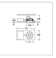
Round emergency luminaire for escape route lighting. With plastic lenses for escape route illumination. Suitable for connection to central battery systems. With AC Control monitoring module for LUXIFAIR central battery units. With enclosed separate ceiling mounting ring also suitable for ceiling cut-outs of Ø 68 mm.
