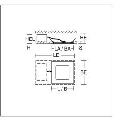
Square recessed downlight. For escape route illumination. Housing: die-cast aluminium, powder-coated. Lightguide and diffuser made of nonyellowing plastic (PMMA). Diffuser opal matt plastic. Ceiling installation with spring system. Including separate LED converter with connecting cable 250 mm. Self-contained system with automatic self-test and feedback to the RZB monitoring system MULTIDIGIT. External driver with simple plug-in locking system.
