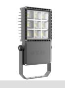
SMART [PRO] 2.0 is a medium power outdoor and indoor LED projector, suitable for lighting sports areas and facilities. It can be installed on the wall, ceiling or ground thanks to the polyester powder coated galvanised steel bracket, with trivalent passivation, equipped with adjustable goniometric scale and supplied in kit. The body is produced in aluminium die casting
