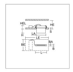
Luminaire for escape route identification. Installation housing sheet steel. Ceiling plate stainless steel high polish or powder-coated. Display panel: highly transparent panel, plastic, with legend on one side/both sides. Electronic ballast included. Self-contained system with automatic self-test and feedback via DALI bus, only to RZB DALI monitoring system. Please indicate legend number when placing your order!
