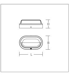
Decorative surface-mounted luminaire for outdoor use. Housing made of corrosion-resistant die-cast aluminium, seawater resistant powder-coated. With membrane valve to avoid condensation. Crystal glass: matt inside. Shadow-free, homogeneous and soft illumination. With mains voltage LED module. Fixing on the wall outside the sealed volume, drill hole deviations can be compensated. Separate connection compartment for direct connection of rigid cables up to 3 x 2.5 mm<sup>2</sup>.
