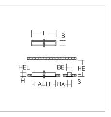
Recessed ceiling and wall luminaire with slim design. Housing: extruded aluminium profile, powder-coated. End cap aluminium powder-coated. Diffuser made of non-yellowing plastic (PMMA), opal. Suitable for Recessed ceiling mounting, wall (recessed). External driver with connecting cable.
