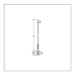
Conical steel pole, according to DIN EN 40. Hot-dip galvanised in compliance with DIN EN ISO 1461. Flush pole door, 85 x 400 mm. Triangular lock, other locks on request. C-slot with two sliding nuts M6 and earthing thread M8. Cable hole 50 x 150 mm (UKK 500 mm below level).
