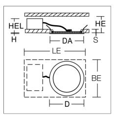
Ultra thin recessed downlight. For escape route illumination. Housing: die-cast aluminium, powder-coated. Lightguide and diffuser made of non-yellowing plastic (PMMA). Diffuser opal matt plastic. Ceiling installation with spring system. Including separate LED converter with connecting cable 250 mm. Self-contained system with automatic self-test. External driver with simple plug-in locking system.
