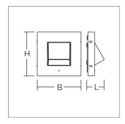
Wall luminaire for escape route illumination. Base: die-cast aluminium, powder-coated Cover: polycarbonate. With plastic lenses for area lighting. Vertical swivel. Electronic ballast included. Self-contained system with automatic self-test. Luminaires with limited surface temperature in accordance with EN 60598-2-24 for use in environments in which a deposit of conductive dust on the luminaire can be expected.
