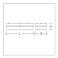
All-plastic luminaires, shockproof. For escape route identification or escape route illumination. Base: plastic (polycarbonate). Refractor: plastic (polycarbonate), transparent, prismatic. 4 legends for escape route identification included. Suitable for Wall (surface). Pendant luminaire also possible with accessories. Suitable for connection to central battery systems.
